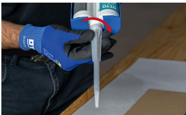
Clean off material and screw on static mixing nozzle
