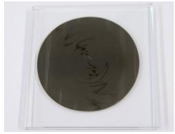
Glass plate test – Expected mixing pattern during cartridge processing
