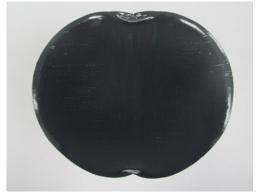
Mixing pattern to be expected when processing using a mixing and dosing system
