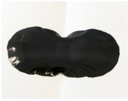
Pull paper apart - Expected mixing pattern during cartridge processing
