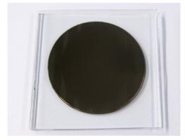
Glass plate test – Mixing pattern to be expected when processing using a mixing and dosing system
