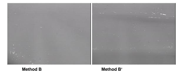
Photo 2: Material **OTTOSEAL® S 68, color white** (at a magnification of x 50) after an incubation period of 28 days (method B and B') without fungal growth
