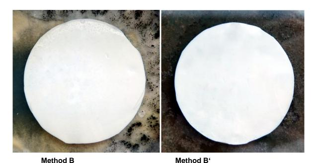
Photo 1: Material **OTTOSEAL® S 68, color white** after an incubation period of 28 days (method B and B') without visible fungal growth
