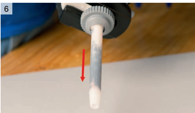
6 Fill the static mixing nozzle with adhesive. Check the homogeneity of the mixture (see quality controls during processing of 2K products).
