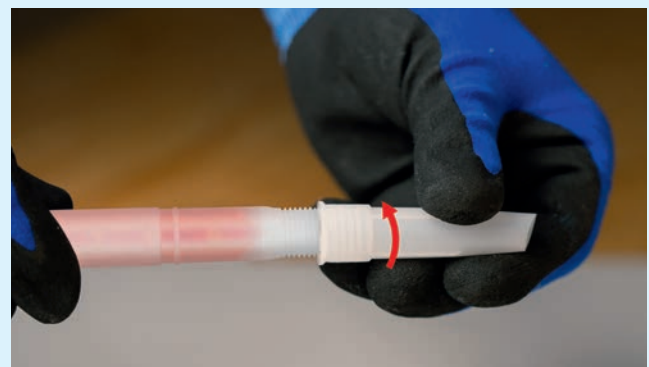
Screw the standard cartridge nozzle onto the static mixing nozzle for BlueLine cartridges as far as it will go
