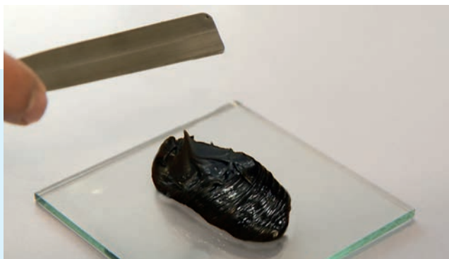
Consistency is 'chewing gum-like', the sealant 'retracts' – pot life has been reached
