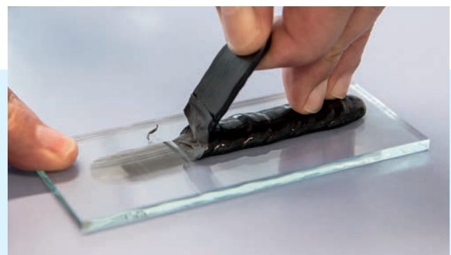
Pulling off the adhesive bead and assessing the fracture pattern: If there is a cohesion break in the adhesive, the adhesion to the substrate is perfect
