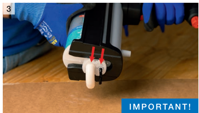
Extrude material without a static mixing nozzle until material emerges from both openings
