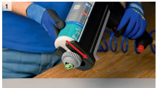
Inserting the BlueLine cartridge into the gun
