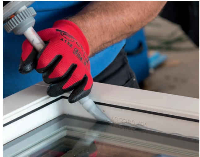
Manual processing of OTTOCOLL® S81 with the BlueLine cartridge
