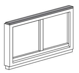
Step 3: Stick the OTTOTAPE Trio-BKA MF1 on the top of the frame. Here the tape is to be cut to the exact length of the top of the frame.
