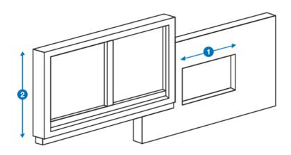
**Step 1:** Determination of the joint width and the joint area. To do this, measure the masonry opening and window frame. The masonry must have a smooth finish and the resulting joint width must match the joint area of the selected multifunctional sealing tape all around.
