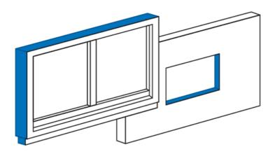
Step 2: Cleaning the window frame and reveal from dirt, dust or other impurities.
