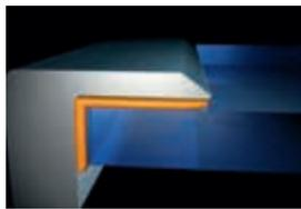
Generally speaking bonds on glass ceramic surfaces are realised with two-part silicone adhesives, which – contrary to “open sealing” – do not have to meet high aesthetic demands because they remain hidden from the end consumer.
